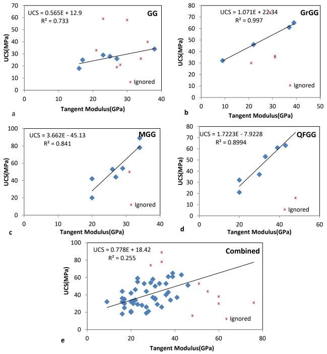
Fig.1 Relationship between Tangent Modulus and UCS for each variant of GG (a-d) and for combined GG (e)
