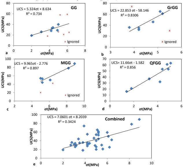
Indirect Tensile Strength (σt) vs Uniaxial Compressive Strength (UCS):
